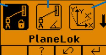
Select **Service**; buttons **6/7** toggle between **Calibration Y** and **Cal X** OR **Cal Z** when set up vertically. Special Field calibration instructions are available.
